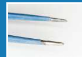
Damaged coating at tips
