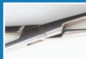
Cracked box joint
