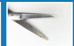
Damage to scissor blade edge
