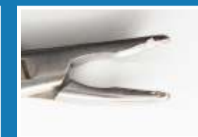
Damage to cutting edge of ronguer
